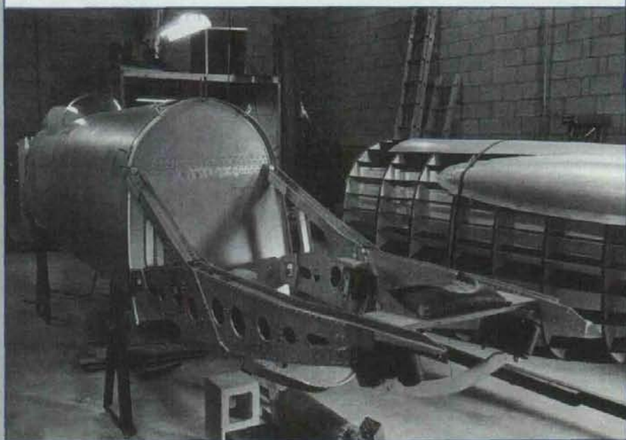
Tsunami's fuselage in 1984. The bed-type engine mount is from a P-51, shortened for this application.
